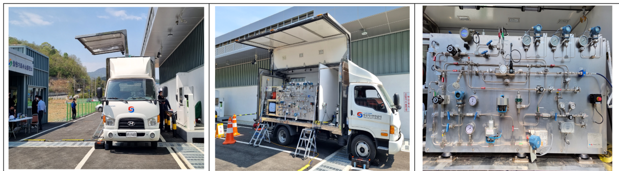
Fig. 1. Vehicle-mounted hydrogen refueling station evaluation equipment (Hy-PAS).
