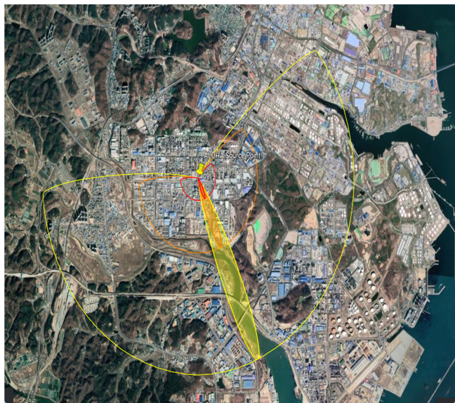
Fig. 6. The result of consequence analysis generated by Aloha in case there is no water curtain operation. (The orange color indicates ERPG-2 zone)
