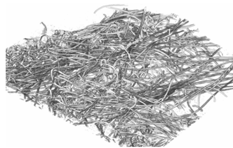
Fig. 2. The microscale image on the conventional nonwoven filter paper used as the hydrophilic membrane, which is made from a mixture of cellulose ( 1.5 \text{ g/cm}^3 ) and polyester ( 1.39 \text{ g/cm}^3 ) with a pore size of around 20 \mu\text{m} .
