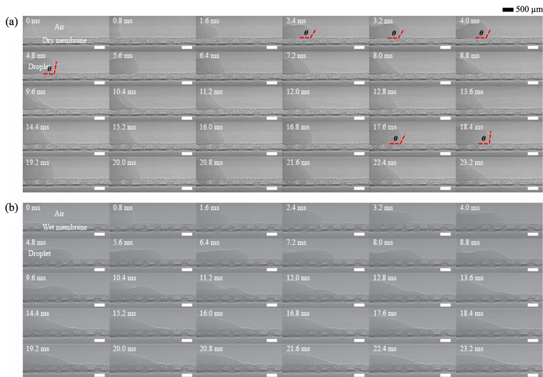
Fig. 3. Transient deformation of spreading of droplets near the contact line on the (a) dry membrane and (b) wet membrane. The scale bar indicates 500 \mu\text{m} .
