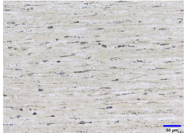
Fig. 2. Surface image of SST-430. Horizontal lines as well as deep scratches were observed, which is typical in case of flat-rolled product.
