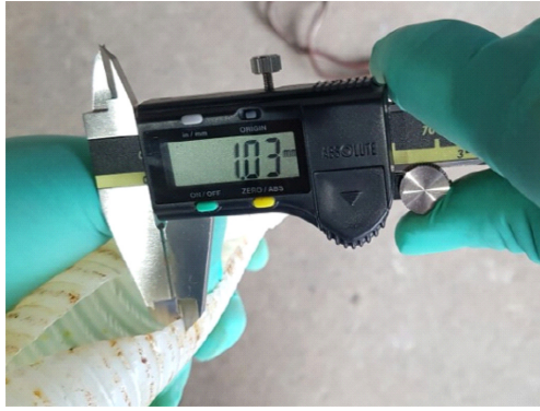
Fig. 4. Flexible hose after deformation.
