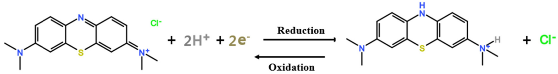
Fig. 1. Scheme of redox reaction of (a) Methylene blue and (b) V^{4+}/V^{5+} .
