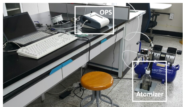
Fig. 4. Constant output atomizer and OPS.
