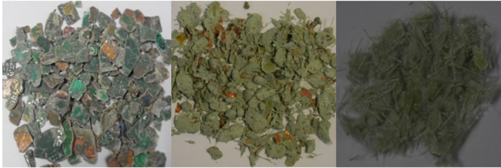
Fig. 2. Waste printed circuit boards (WPCBs) using shredding mill (left); resin, glass fiber and copper (middle) using the three-blade agitator, glass fiber (right) using the attrition mill in the DMF.
