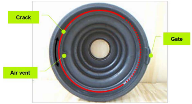
Fig. 2. Locations of cracks observed in the boots produced by K company and the positions of both gates and air vent from its mold design.
