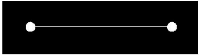
Fig. 1. Pattern of the microchannel (width: 300 μm, depth: 100 μm, length: 40 mm, reservoir diameter: 7 mm).
