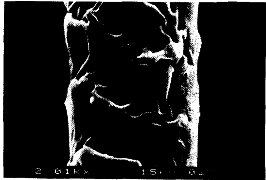
Photo. 1. Photograph of undesorbed wool (×2000).
